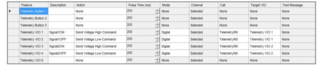
Important settings are Telemetry VIO1-4. Other Telemetry settings can be used for other functions.
