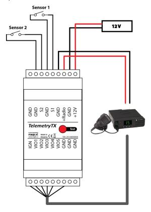
If you have continuous AC power and do not have solar cells then Motorola MotoTRBO radio can be connected to permanent 12V. You can also omit IGN wire from Telemetry TX and connect to +12V.
