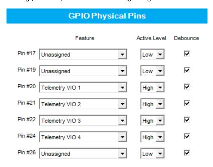
Important settings are for pin #20, #21, #22, #24. Other pins can be used for other functions.
